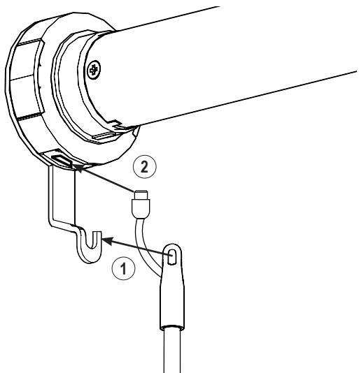
On Banded Shades, Roller Shades and Sheer Shadings, with the wand control buttons facing you, attached the top of the wand on the metal hook support (1) on the motor control side, then connect the cable into the motor head (2).
