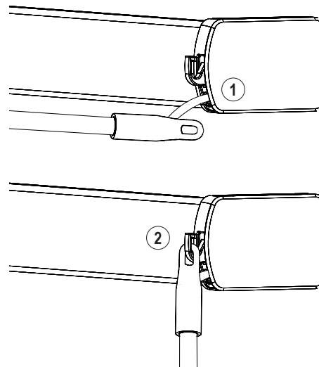
On Honeycomb shades, the wand will be already connected to the shade (1). With the wand control buttons facing you, attached the top of the wand into the plastic hook support on the motor control side (2).
