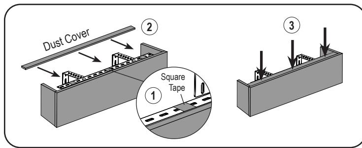
First, remove adhesive backing from square tapes and place the square tapes on slotted angle. Then, put the dust cover on top of slotted angle and press it to secure the adhesive.
