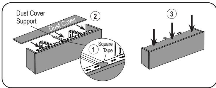
First, snap the dust cover support onto the slotted angle. Then, remove adhesive backing from square tapes and place the square tapes on slotted angle and brackets. Press the dust cover in place to secure the adhesive.
