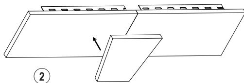
First, place the two or three fabric cornice sections on a straight surface face down and align edge-to-edge. Install splice brackets with provided screws and proceed to step **1. Install the Brackets**. Once the cornice is installed, attach keystone with provided velcro strips at the center, covering the splice.
