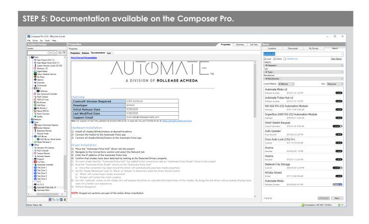
This driver is an Interface Controller for the SHC Pulse Pro Hub. It allows IP control over SHC shades from CONTROL4.
