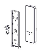
Use supplied fasteners and anchors to attach the base to wall.
